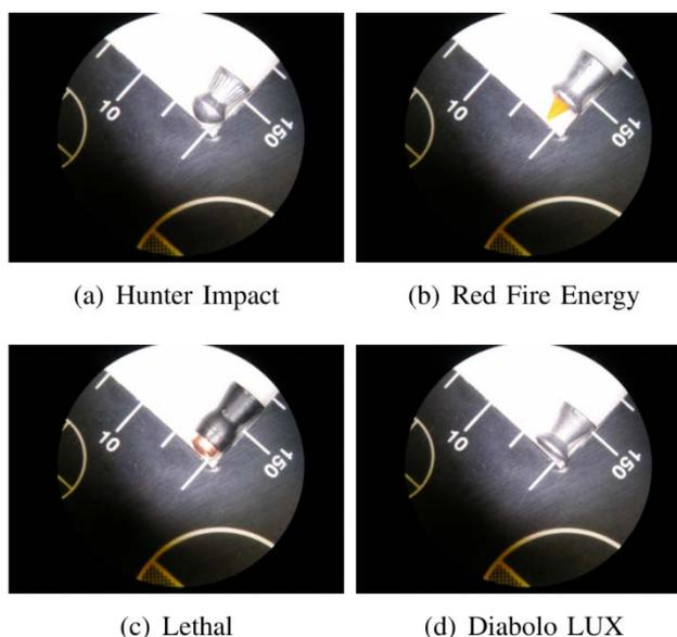
**Figure 2.** Microscopic photos of selected diabolo pellets
