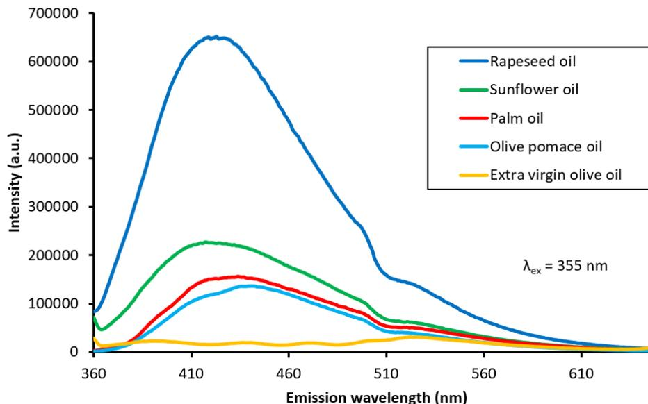
Figure 4. Emission spectra of tested edible oils
