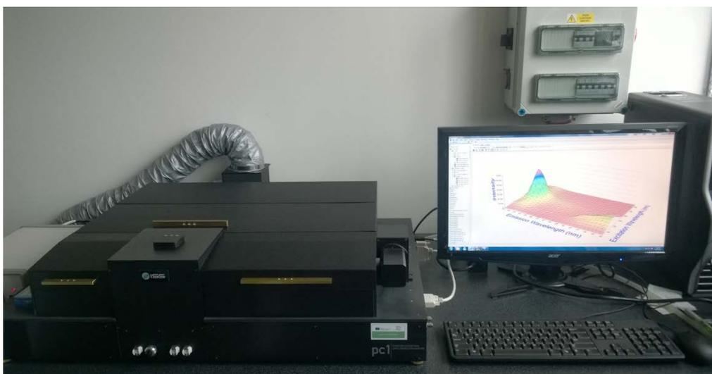
Figure 1. ISS PC1 spectrofluorometer connected to the computer
